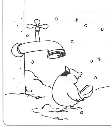
It's freezing cold outside. The water pipes are getting colder and colder. Any water inside the pipes will turn to ice soon. When the water in the pipes freezes, it will take up more space. If the faucet is turned off, there is no more space. The ice may burst the pipes.
